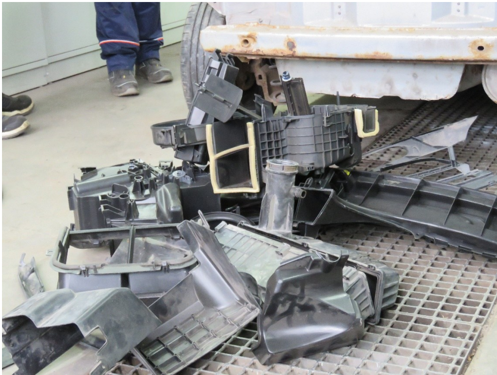
Figure 4. PP-TD and PP-MD components are also found beneath the dashboard. In this case, TD and MD most likely refer to talc-filled and mineral-filled grades.
