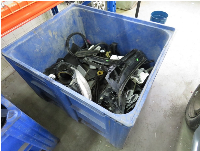
Figure 7. Elastomers and foamed polymers excluded from recycling, as well as multi-material components containing them.
