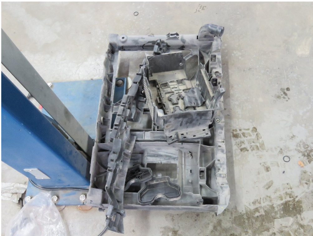
Figure 4. PP-TD and PP-MD components are also found beneath the dashboard. In this case, TD and MD most likely refer to talc-filled and mineral-filled grades.
