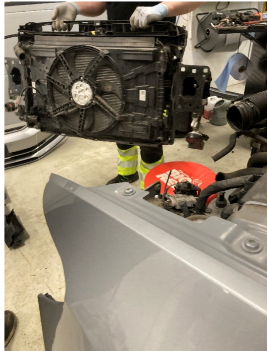
Figure 10. Removal of the rear bumper (left) and front radiator assembly (right)
