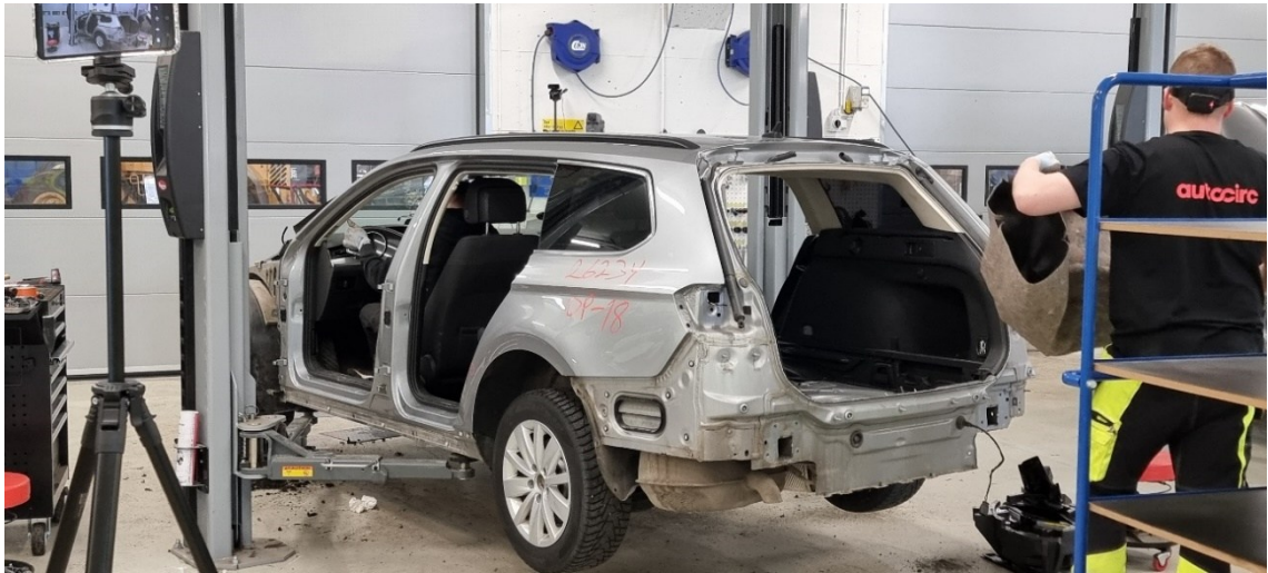
Figure 14. Dismantling of the luggage compartment interior and dashboard work
