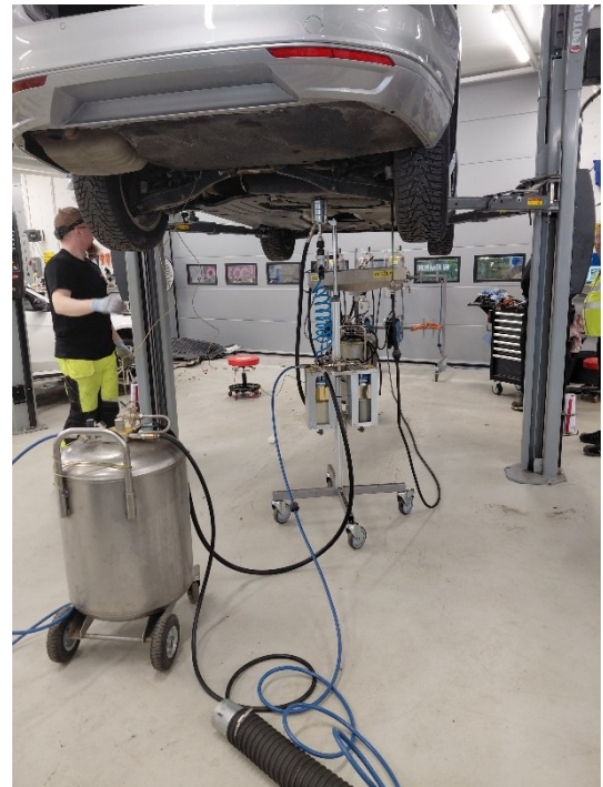
Figure 7. Depollution equipment (left) and fuel extraction system (right)
