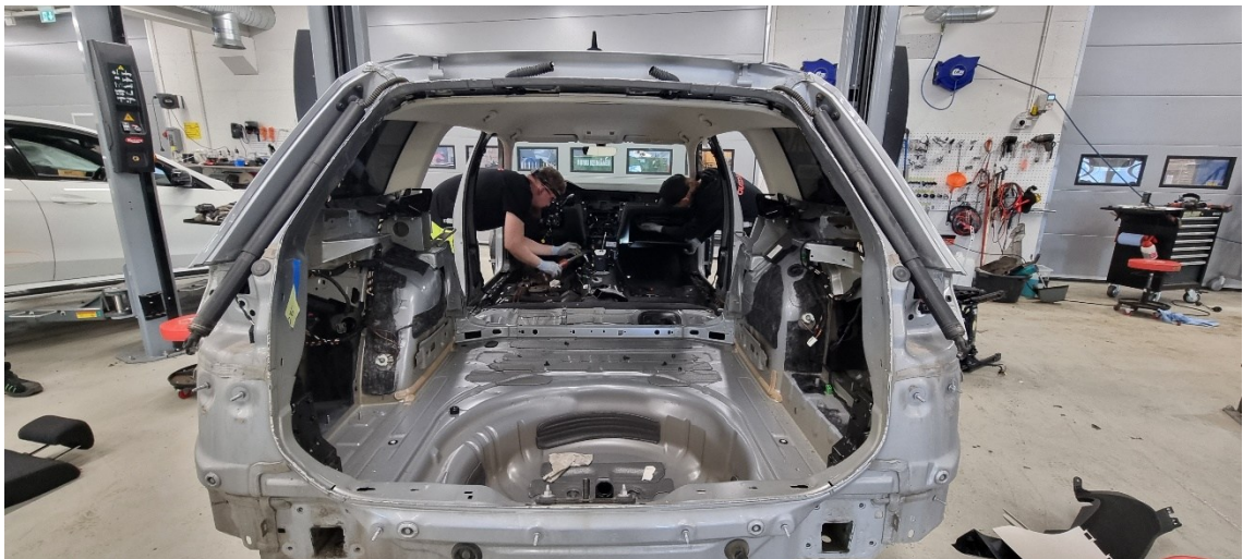
Figure 16. Work on the dashboard and centre console and completion of interior dismantling.
