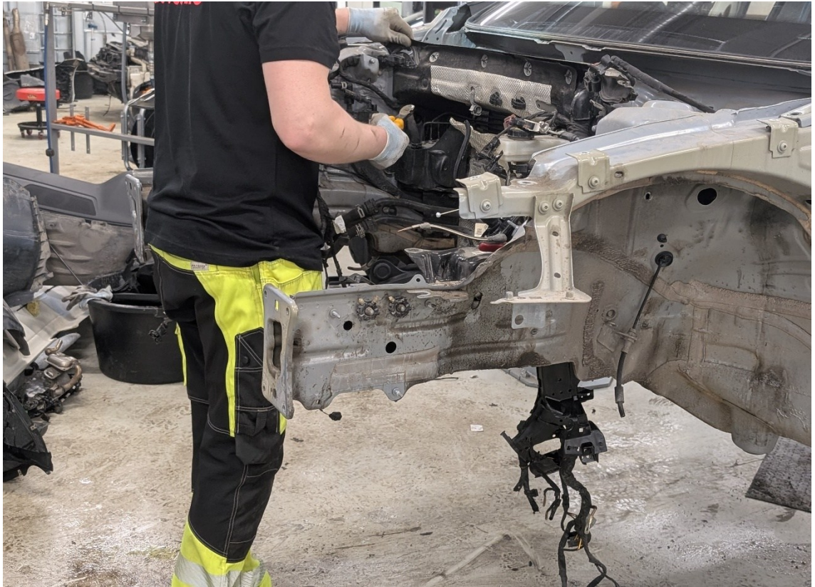
Figure 26. Removal of the engine bay main wiring harness
