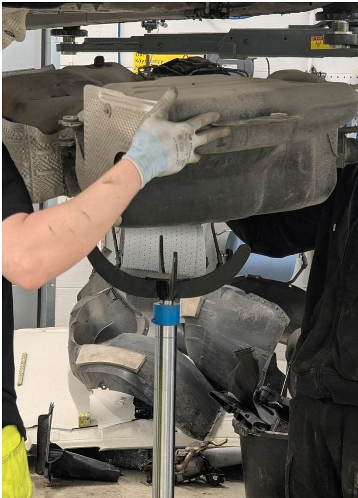
Figure 25. Removal of the fuel tank
