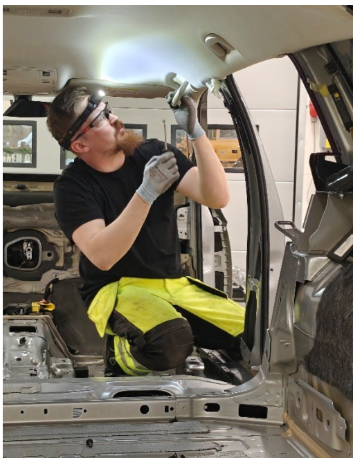
Figure 18. Removal of the grab handle to allow headliner removal (left) and airbag removal (right)
