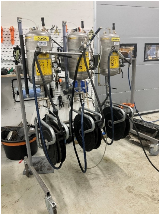
Figure 7. Depollution equipment (left) and fuel extraction system (right)
