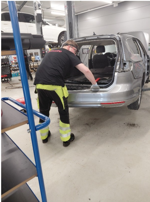
Figure 10. Removal of the rear bumper (left) and front radiator assembly (right)
