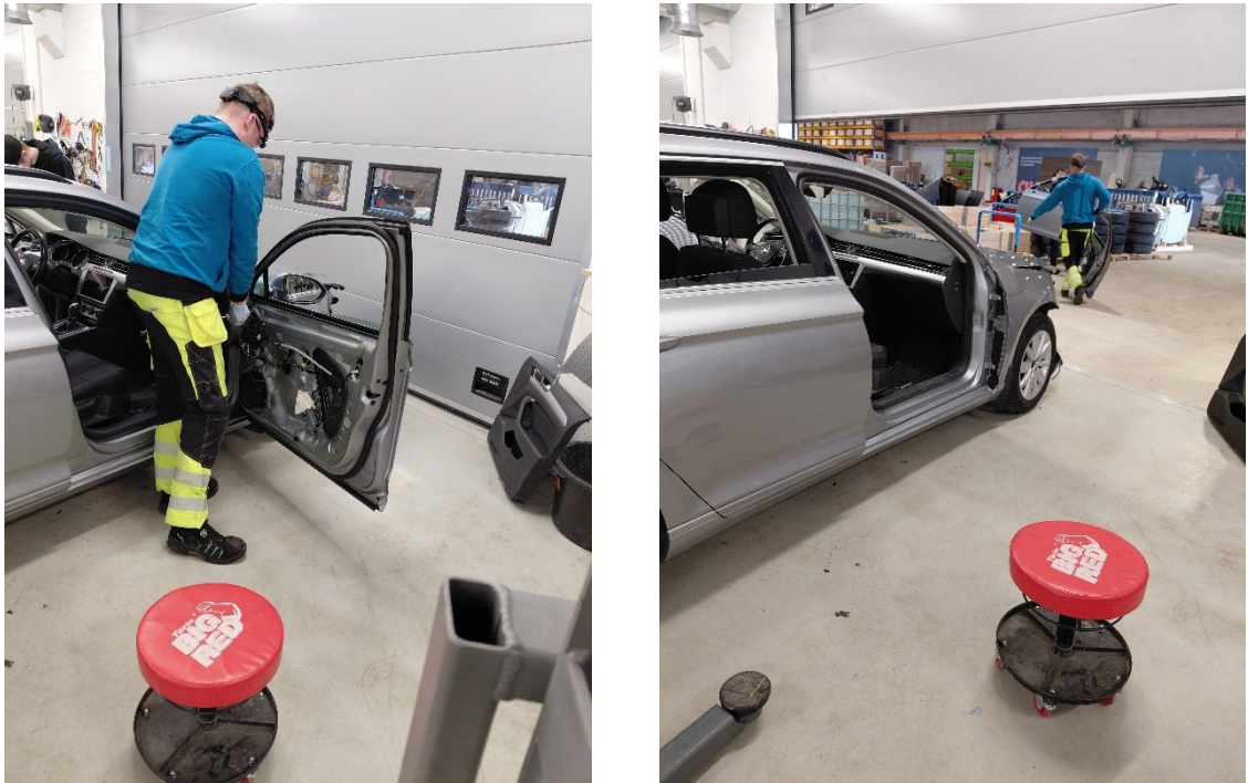
Figure 4. Door removal (left) and transfer from the dismantling area (right)
