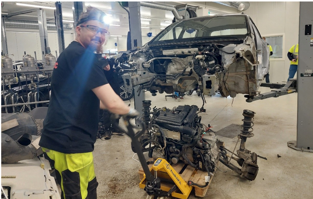
Figure 22. Powertrain and front axle assembly removed onto a EUR pallet
