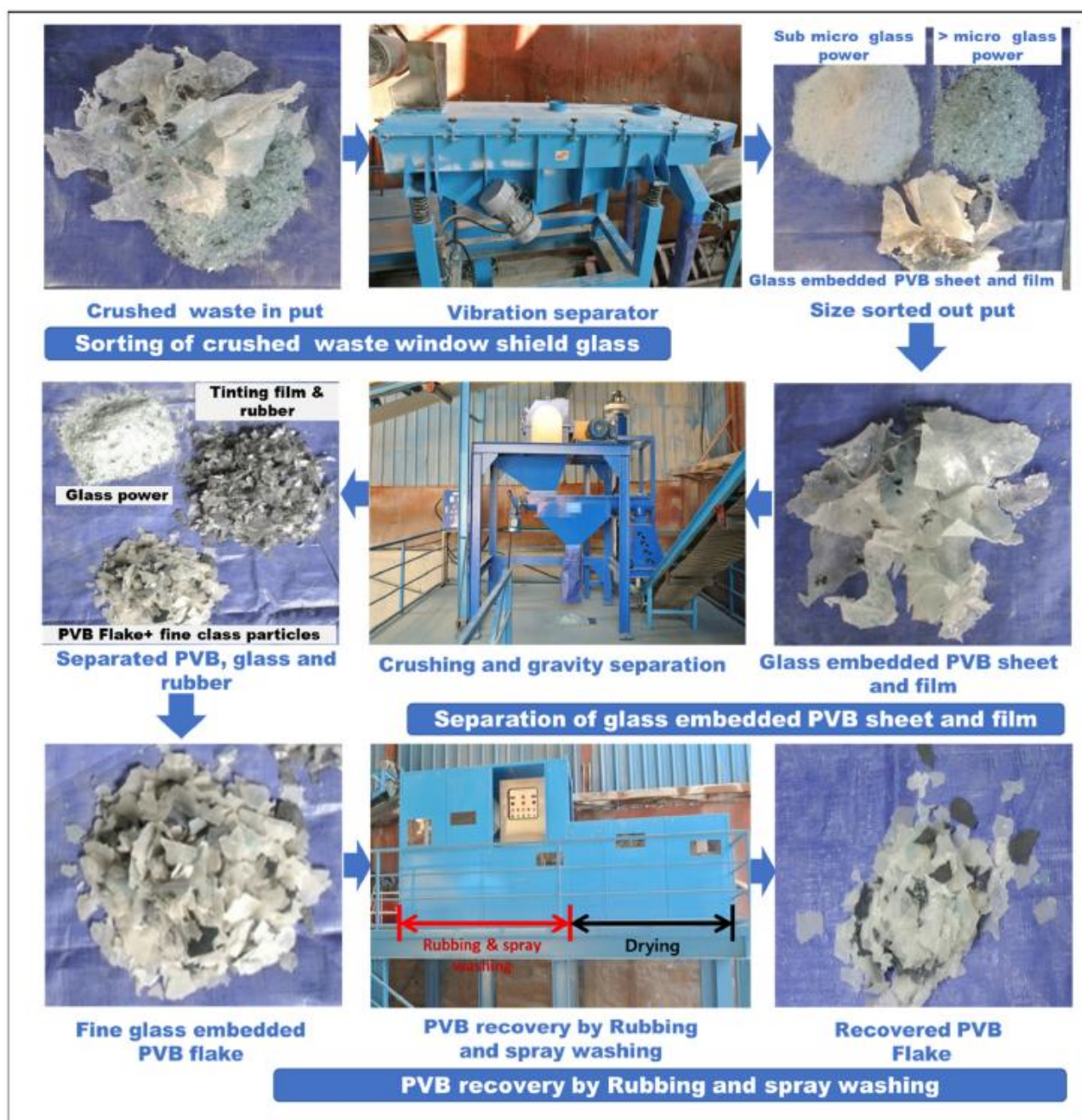
Fig. 5. Mechanical separation and sorting of size reduced ELV windshield glass. The picture presented is not in proportionate scale, dimension reflects in Table 1.
